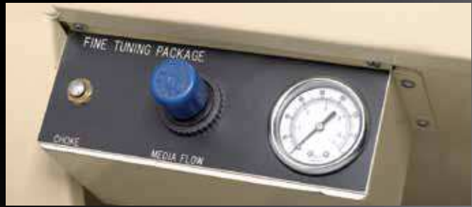
Fine-tuning controls let operator adjust air/grit ratio from cabinet front for optimum results.
