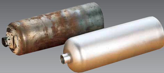
Cylinder surface profiled with aluminum oxide
